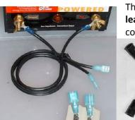
The E-Track and the E-Charger unit are connected using **AVITHOR copper dual lead wire**. This special, highly insulated wire, is available separately. To connect the wire, simply strip the ends of the dual leads and connect the
