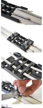
To make a connection, thread the stainless steel braids through the two holes in the Connector and lock the braids in place. The stainless steel braids move current from one track to the next.
